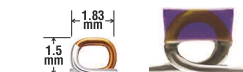
The square shape and narrow footprint reduce board space by 60-75% over conventional air core inductors.
