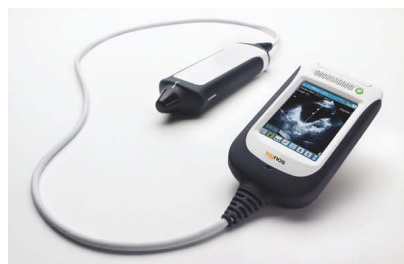
Figure 5 Ultrasound systems are becoming available in handheld form factors (courtesy Signostics Medical).
