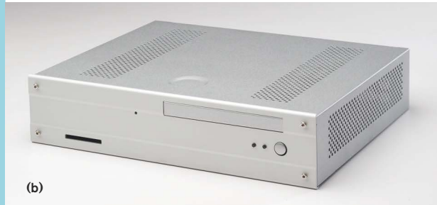
Figure A Combining the 1-GHz fanless-CPU version of Via Technologies' EPIA SN mini-ITX board (a) with a two-drive customized version of Casetronic's Travla C137 enclosure (b) and hard-disk drives from Seagate and Western Digital forms a stable and robust test bed for several NAS operating systems.
